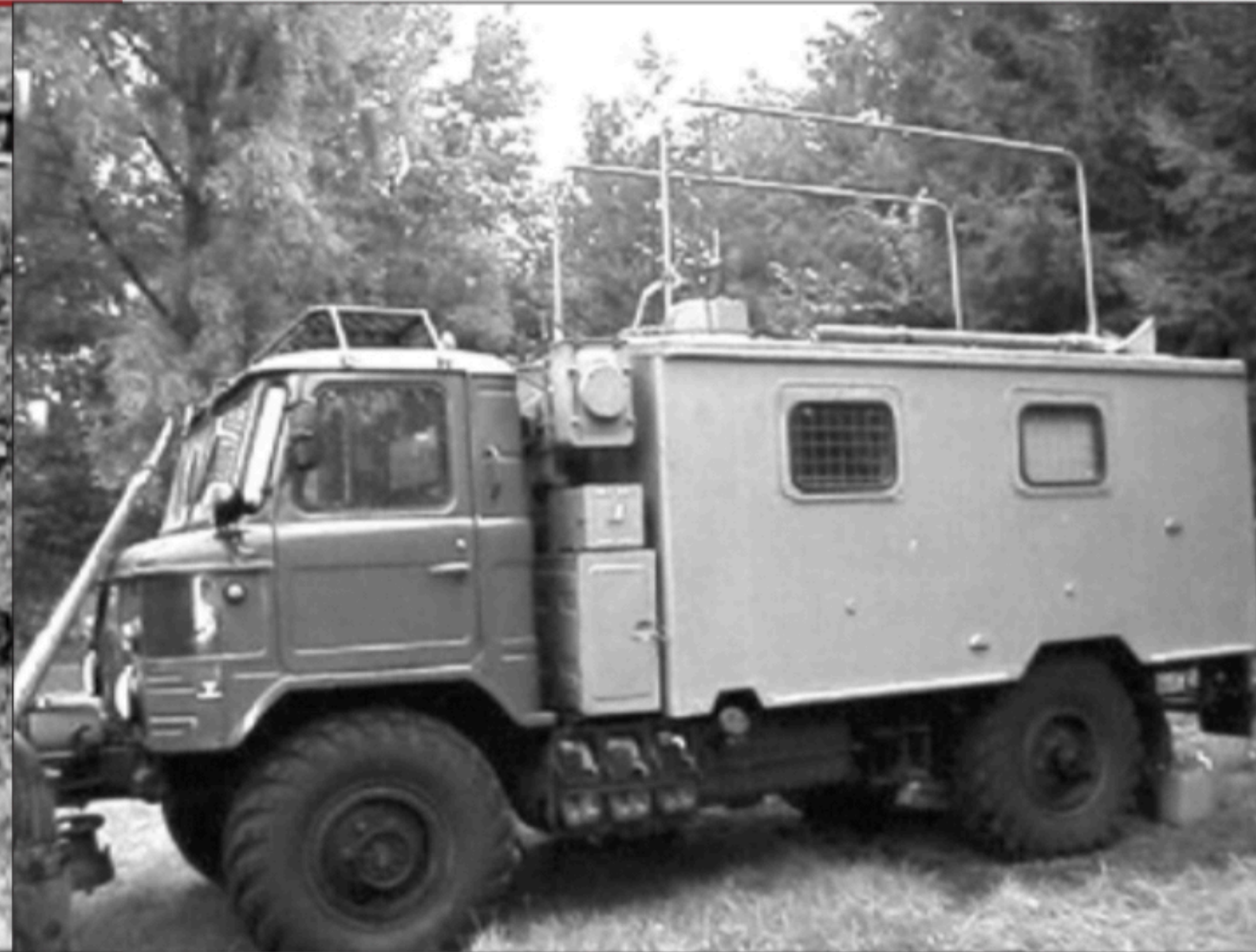
Fig. 9 (Left) A Russian communications vehicle with two vertical loop elements.
